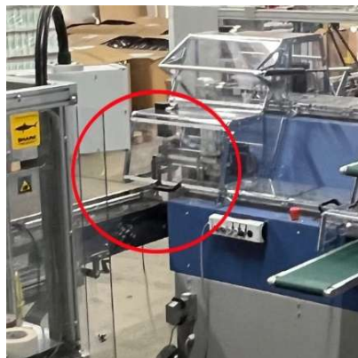
15) Interface to e.g. cellophane wrapping machine
