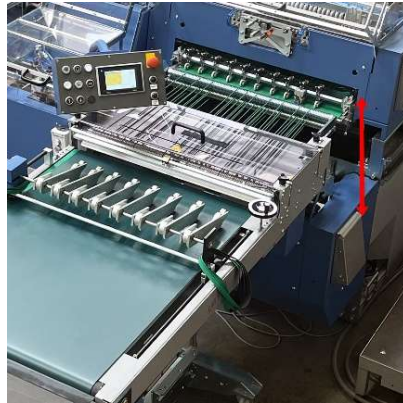
13) Lowerable collecting station for subsequent machines such as Stream Deliveries or Stackers
