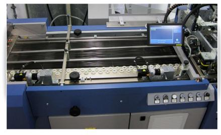
The camera system measures the distances between the sheet edge and the print mark on each individual sheet. The dynamic side alignment corrects the determined differences.
