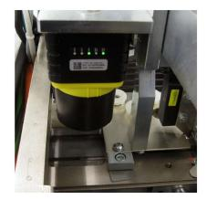
The differences determined by the camera are transmitted to the controller
