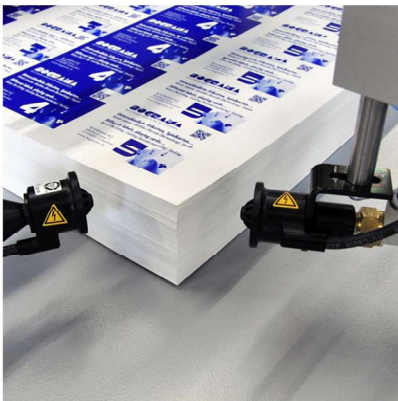
Discharge nozzles at the feeder
