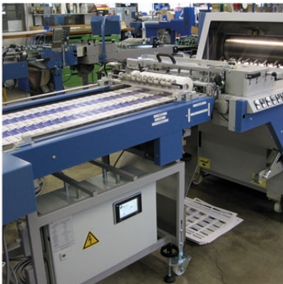
Stream belt 550 in connection to BSR 550 Servo with new breakout unit
