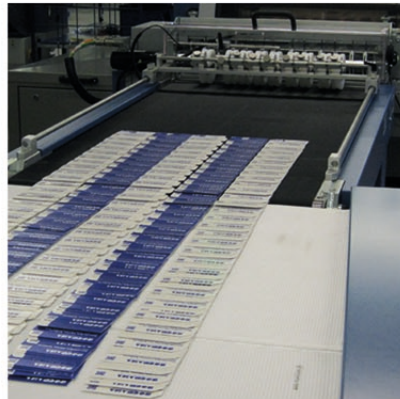
Direct delivery of the shingled products to the stream-spreading conveyor
