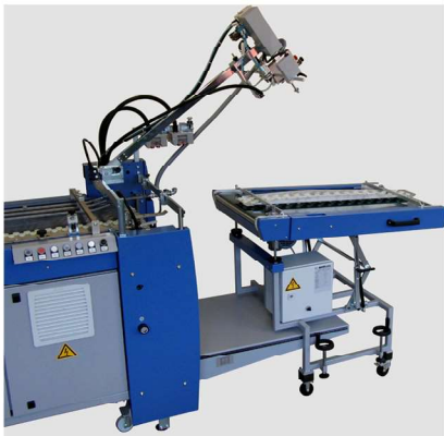
Simple changeover; lower the table, lift the feed head and position the ULT 550
