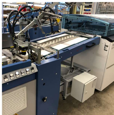
Inline configuration BSR 550 Servo with ULT 550 and cross cutter
