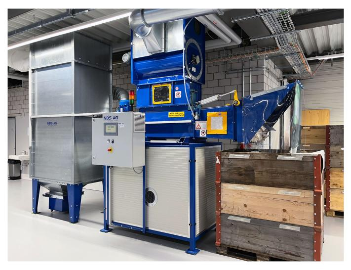
Extraction unit for paper cuttings and dust. The dust-laden air is freed from dust and returned in production areas cleanly.
