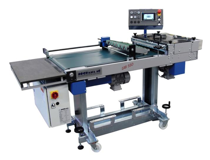
The SAB 550 / 750 stream delivery is used for multiple-up production. Formats from A3 to 35 x 35 mm (minimum) can therefore be delivered in streams
