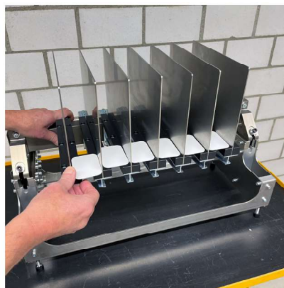
The side plates of the stacking shaft can be set to size outside the stack delivery
