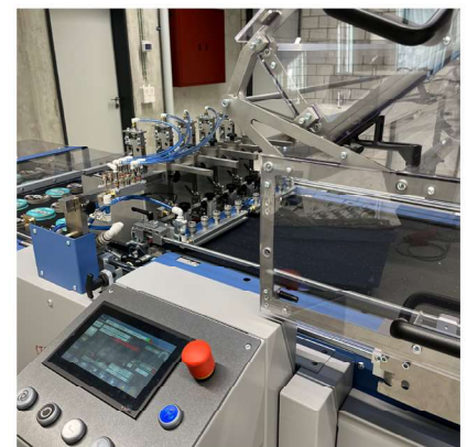
Vacuum belt for stable transport in a shingled stream or as individual products
