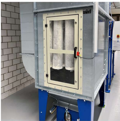
Filter unit for cleaning and recirculation of dust-laden air
