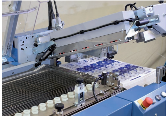
Flat pile feeder with Tornado vacuum modules
