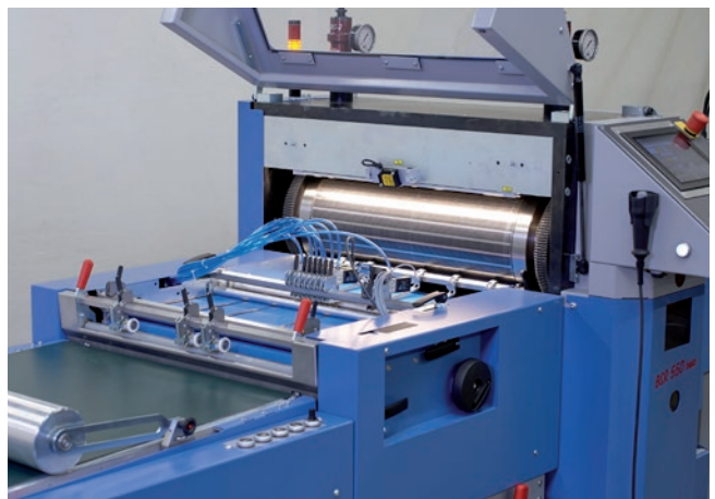
Breakout and deliver unit, adjustable without tools
