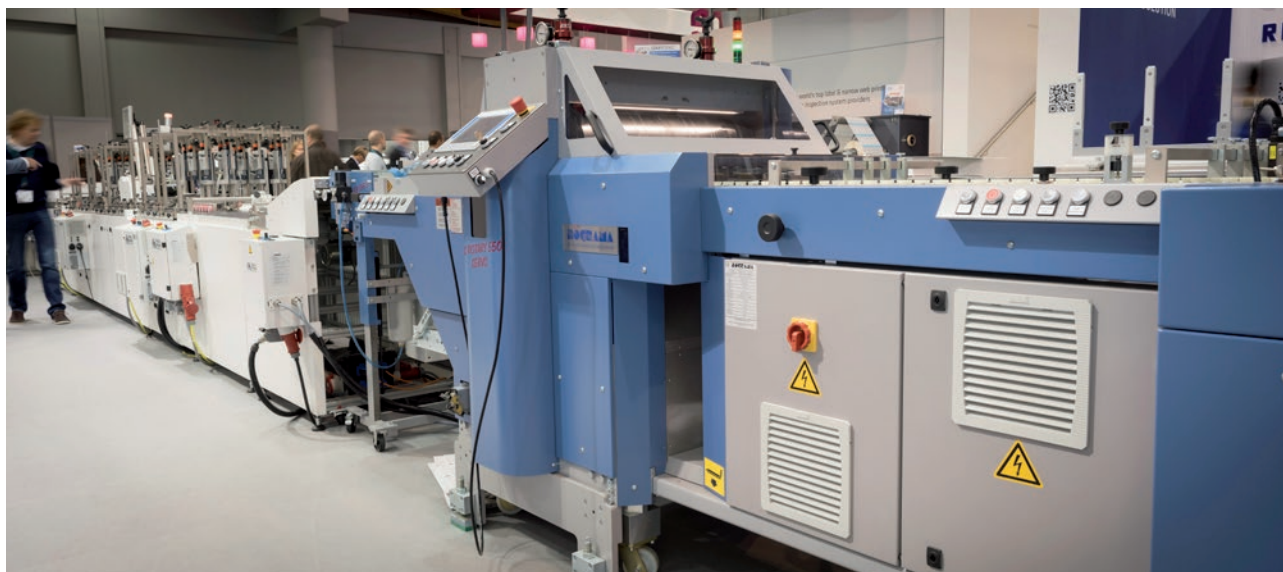
Packaging-Line „Stamina“, consisting of BSR 550 Servo with pallet feeder and Herzog + Heymann folding carton line.
