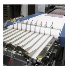
SSB 550 Stream-spreading conveyor, for inline production with BSR 550 Servo rotary die-cutter
